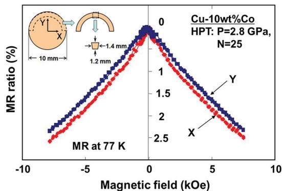
Figure 10. Variation of MR ratio with magnetic field in two different directions ( $X$  and  $Y$ ) for HPT sample after  $N = 25$  revolutions, where the definition of  $X$  and  $Y$  is as illustrated.[102]
