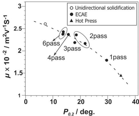
Figure 21. Dependence of carrier mobility  $\mu$  on preferred orientation angle  $P_{0,2}$ , after applying different numbers of passes of Route A ECAP (labeled ‘EACAE’ in the original figure (from [148])).
