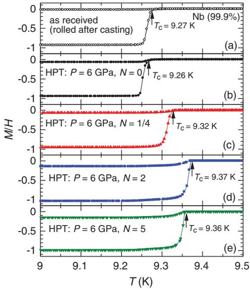
Figure 18. Temperature dependence of the magnetization  $M(T)$  of Nb in the magnetic field  $H = 2$  Oe. (a) As-received sample; (b)–(e) HPT-processed samples with different revolution numbers  $N$ . [141]
