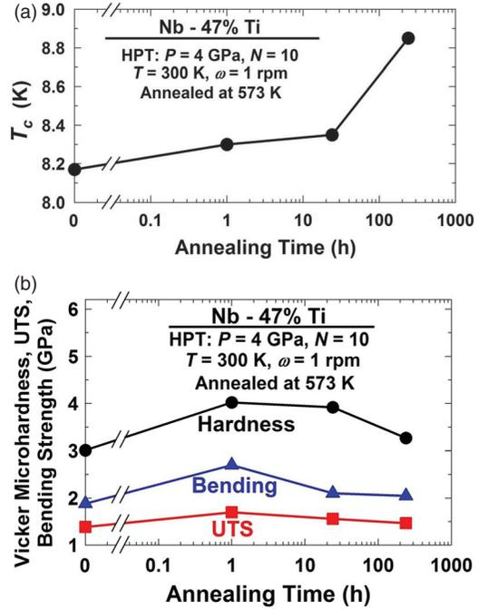
Figure 19. Variation of (a) transition temperature for superconductivity,  $T_c$ , and (b) Vickers microhardness, UTS, and bending strength against annealing time for samples processed by HPT for  $N = 50$  turns and annealed at 573 K. [143]
