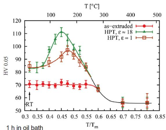
Figure 27. Microhardness of samples of  $Mg_{0.2}Zn_{0.5}Ca$  as a function of homologous annealing temperature  $T/T_m$  ( $T$  and  $T_m$  denoting the annealing temperature and the melting temperature in Kelvin, respectively): (i) after 1 h annealing (full circles) and (ii) after HPT processing and annealing (squares and triangles). HPT processing was done at a pressure of 4 GPa up to von Mises equivalent strains  $\epsilon$  indicated.[183]
