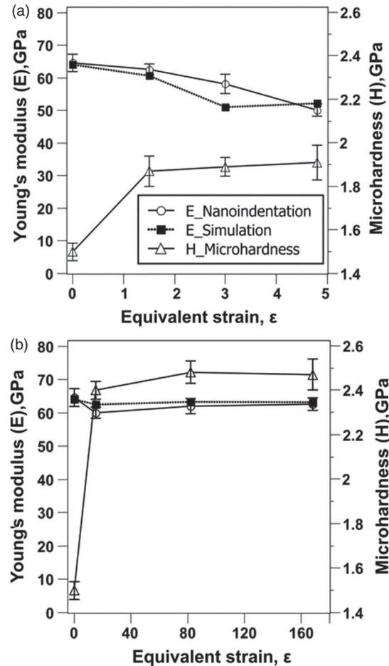
Figure 26. Young's modulus  $E$  as measured by nanoindentation (open circles), and microhardness  $H$  (open triangles), as a function of von Mises equivalent strain  $\epsilon$ , for R & F (a) and HPT samples (b). The values of  $E$  were also calculated from texture data (full squares).[168]
