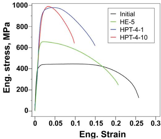
Figure 25. Stress–strain curves for initial and SPD-processed Ti-45Nb samples. HE-5 stands for 97% area reduction by HE, HPT-4- $X$  for High-Pressure Torsion at a pressure of 4 GPa and  $X$  revolutions.[168]
