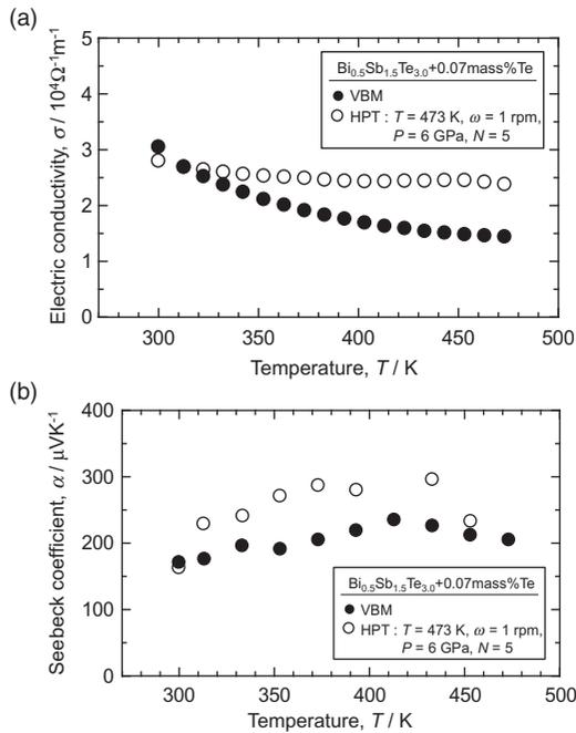
Figure 20. Electrical conductivity (a) and Seebeck coefficient (b) vs. temperature, for  $p$ -type  $\text{Bi}_{0.5}\text{Sb}_{1.5}\text{Te}_{3.0}$  after processing by the Vertical Bridgman Method and HPT.[147]
