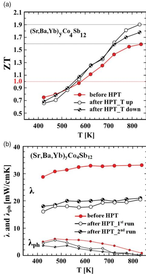
Figure 23. (a) Increase in ZT to a world record  $ZT = 1.9$  by HPT processing; the increase is mainly due to the decrease in thermal lattice conductivity  $\lambda_{\text{ph}}$  shown in (b) [151]
