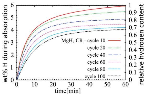
Figure 14. Hydrogen absorption of MgH<sub>2</sub> after cold rolling at room temperature after different numbers of cycles of hydrogen loading and unloading, according to [108].
