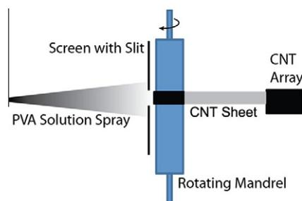
**Fig. 1 – Schematic view of spray winding. A CNT sheet is drawn out of a drawable array and continuously wound onto a rotating mandrel on which micrometer-sized droplets of PVA solution are deposited. A screen with a slit is used to control the spray area.**
