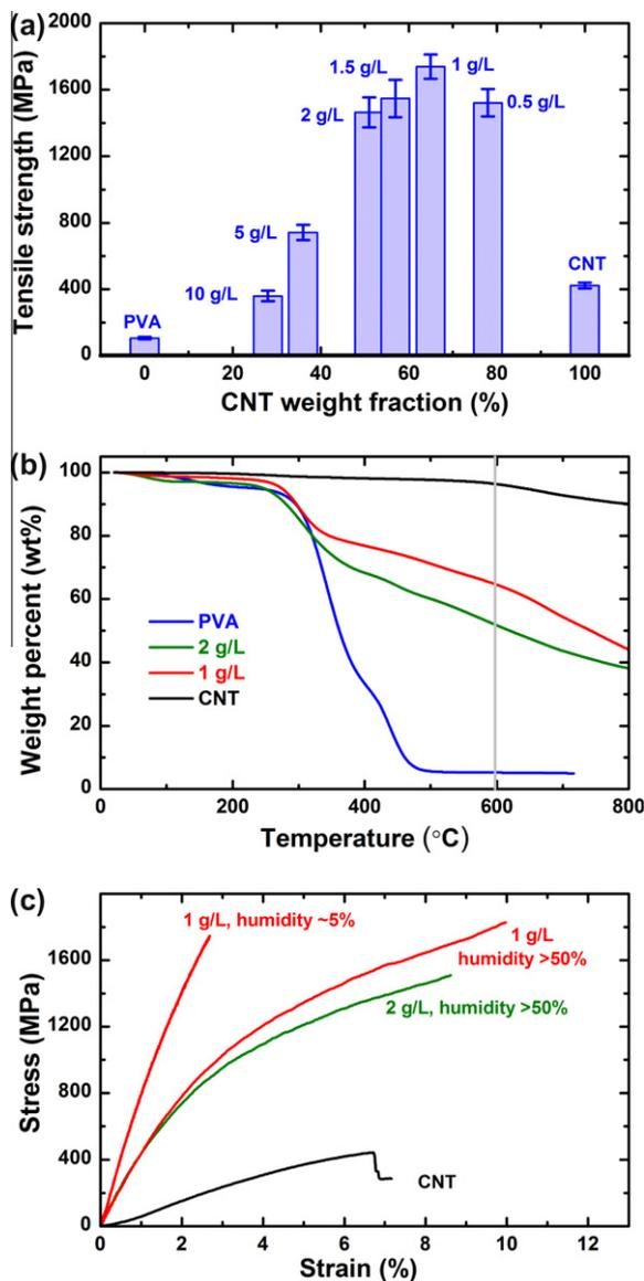
**Fig. 2 – (a) Tensile strength of the CNT/PVA composites as a function of the CNT weight fraction. The corresponding concentrations of PVA solutions are labeled. (b) TGA curves for a pure CNT film, two CNT/PVA films, and a pure PVA film. The fraction in a film was estimated by using the TGA results at 600 °C, similar to Liu et al. [20]. (c) Stress–strain curves of a pure CNT film and three CNT/PVA films, under different ambient humidity.**
