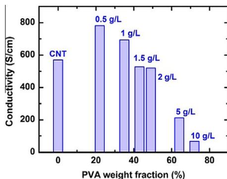
Fig. 5 – Electrical conductivities of CNT/PVA composites as a function of the PVA weight fraction.
