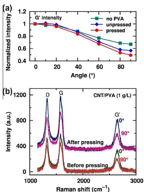
**Fig. 3 – (a) Normalized intensity of  $G'$ -band peak versus the angle between the sample's longitudinal direction and the polarization axis of the incident laser beam. The normalized intensity at  $90^\circ$  becomes smaller when PVA is introduced into the composites, and further decreases after the hot pressing. (b) Raman spectra at  $0^\circ$  and  $90^\circ$ , before and after the hot pressing. All the composite films were produced by using the 1-g/L PVA solution.**
