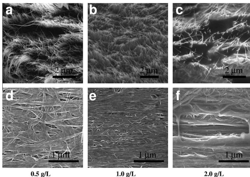
Fig. 4 – SEM images of the cross-sections (a–c) and the top views (d and f) of CNT/PVA films produced by using the 0.5-, 1-, and 2-g/L PVA solutions. For a small PVA fraction, large empty spaces can be observed either between different CNT layers (a) or between CNTs in the same layer (d). In contrast, over-spraying of PVA led to excessive matrix around the CNTs (c and f).
