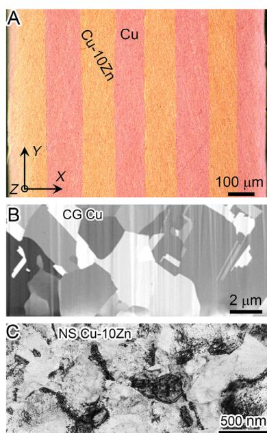
**Fig. 1.** Microstructure of laminate: (A) an optical image showing the stacking of Cu and Cu-10Zn layers, (B) ICCM image of the Cu layer, (C) TEM image of the Cu-10Zn layer. In the coordinate, Y is the rolling as well as the tensile loading direction, and X is the layer thickness direction.
