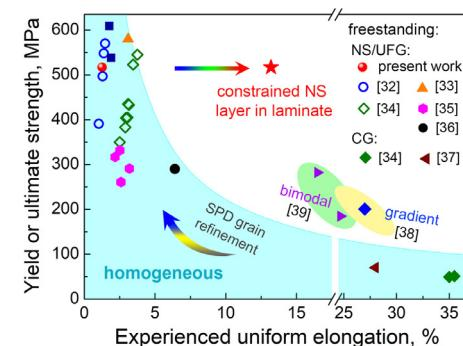
**Fig. 3.** The combination of strength and uniform elongation of the constrained NS layer in laminate, in comparison with the freestanding brasses (with 4.6–11wt.%Zn) characterized by conventional homogeneous microstructure or newly designed heterogeneous microstructure. The data of yield strength and ultimate strength are presented by solid and open symbols, respectively.
