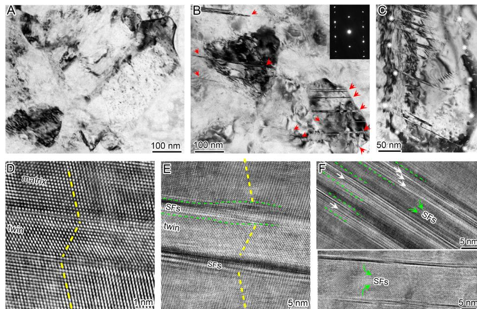
**Fig. 5.** TEM images of the constrained NS layer (A) before and (B-F) after tensile deformation. (C) An elongated grain, in which the white dots indicate grain boundary. (D-F) High resolution images taken from the grain shown in (C), showing the deformation twins and stacking faults (SFs). The red arrows in (B) indicate the nanotwins. The green lines in (E) and (F) mark the regions with high-density SFs.
