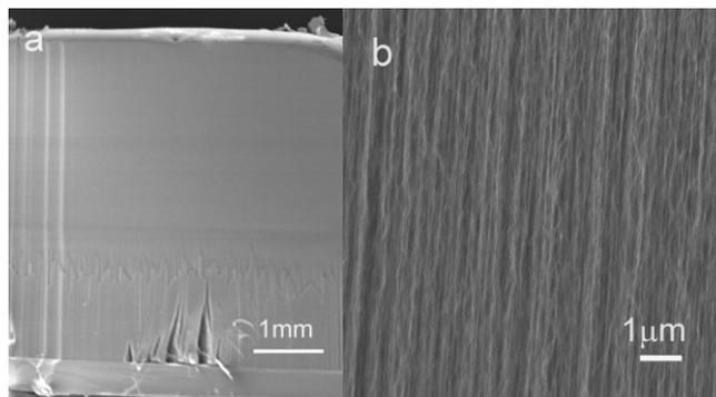
**Figure 1.** a) 4.7 mm long CNT arrays grown on the catalyst  $\text{SiO}_2/\text{Al}_2\text{O}_3(10\text{ nm})/\text{Fe}(1\text{ nm})$  with the assistance of water vapor. b) Enlarged SEM image showing well-aligned CNTs.
