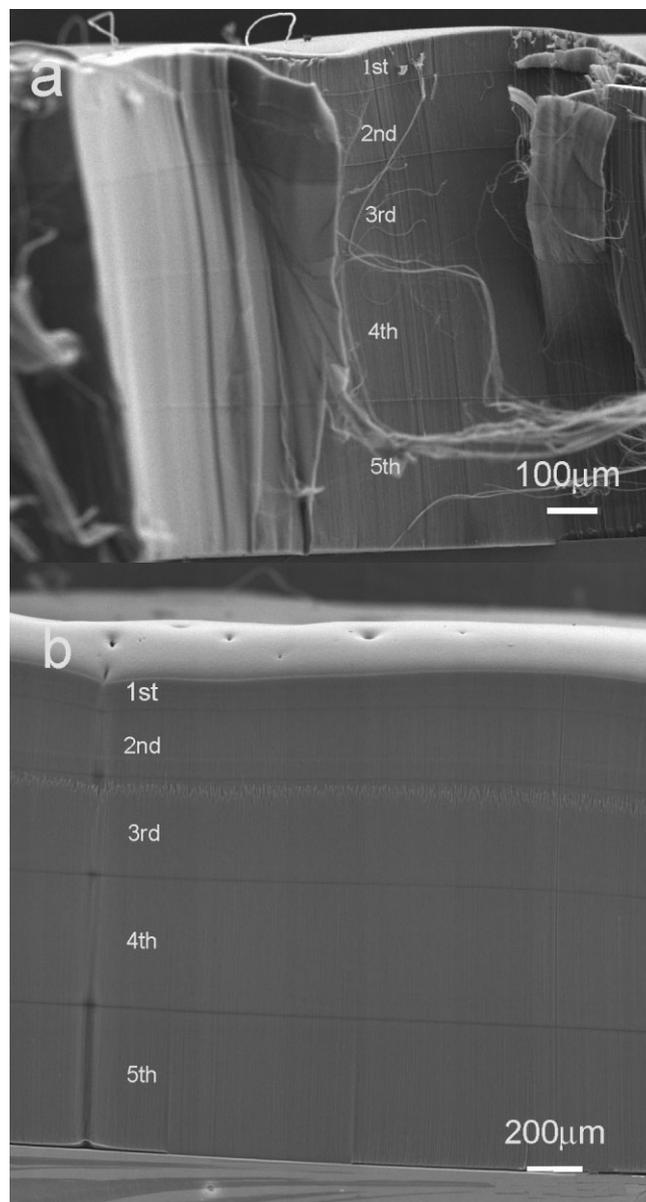
**Figure 4.** a) SEM image showing growth marks formed at  $750^\circ\text{C}$ , without water vapor. b) Growth marks formed at  $780^\circ\text{C}$ , with water vapor. The presence of growth marks on both samples indicates a base growth mode on this catalyst. The numbers indicate the sequence of the injections.
