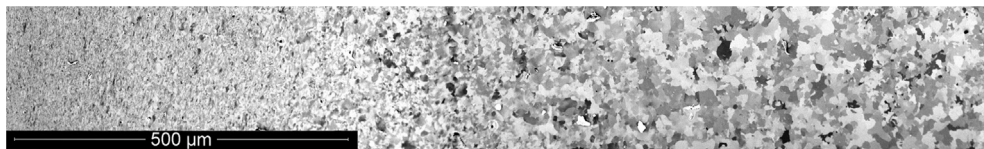
Fig. 60. Schematic illustration of microstructural characteristics along the depth in the surface layer subjected to SMAT.
